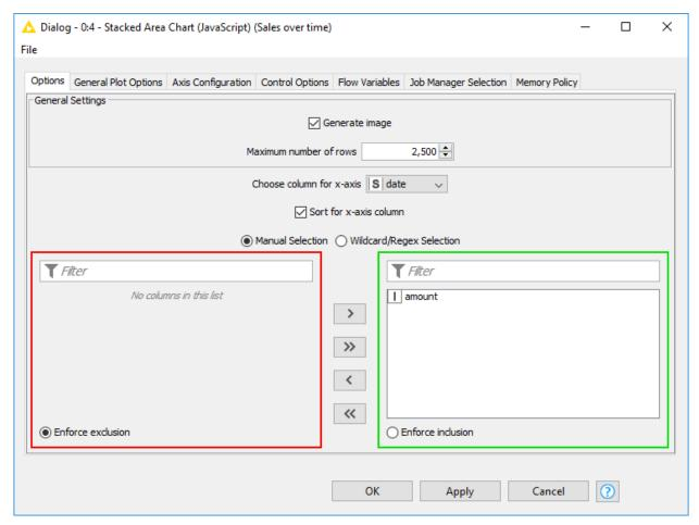
Figure 11. Configuring the Stacked Area Chart node
