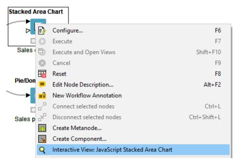
Figure 15. Opening interactive view of an executed node
