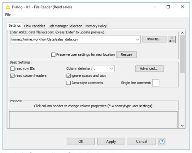
Figure 8. Configuration dialog of the File Reader node
