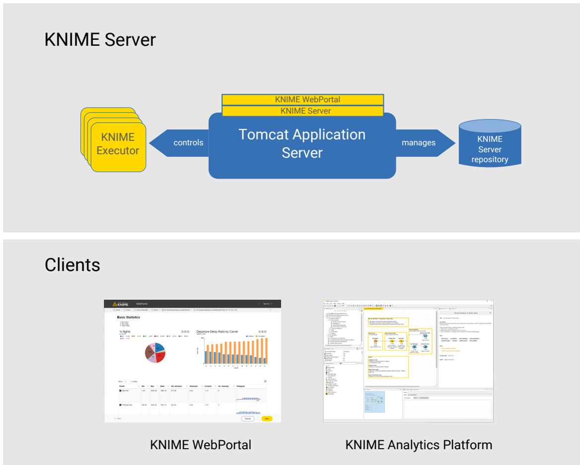
One of the main tasks of KNIME Server is to manage and control the server's repository. Workflows uploaded to the server go through the server application and are stored in the repository which is just a folder on the server's file system (the blue cylinder on the right in the diagram). Access to the stored workflows is controlled in KNIME Server and access rights for the workflows can be manipulated from KNIME Explorer once the client side server extensions are installed.
