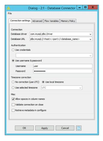
The generic *Database Connector* node can connect to arbitrary JDBC compliant databases. The most important node settings are described below
