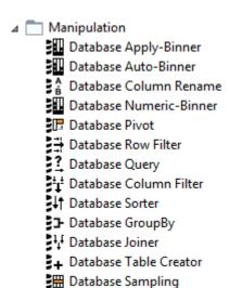
Once you have successfully connected to your database, there is a set of nodes that provide **in-database** data manipulation, such as row filtering, joining etc.
