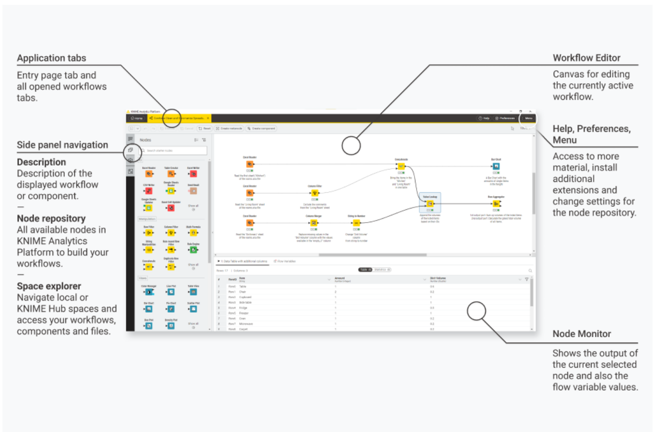
Figure 3. General user interface layout – application tabs, side panel, workflow editor and node monitor
